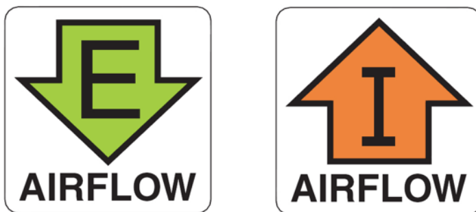
FIGURE 42 Examples of airflow symbols
